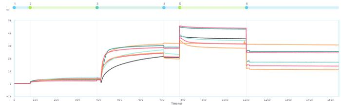
**Figure 2:** Activation of response channels with EDC/NHS from Nicoya's Surfacing Kit, followed by immobilization of 40 µg/mL ProA in Sodium Acetate pH 5.0, 25 µg/mL VHH-EGFP in Sodium Acetate pH 5.5, 20 µg/mL of IL-6R in Sodium Acetate pH 5.0 and 30 µg/mL of IgG2A in Sodium Acetate pH 5.5 and blocking of sensors with 1 M Ethanolamine. Image was generated by Nicosystem analysis software.
