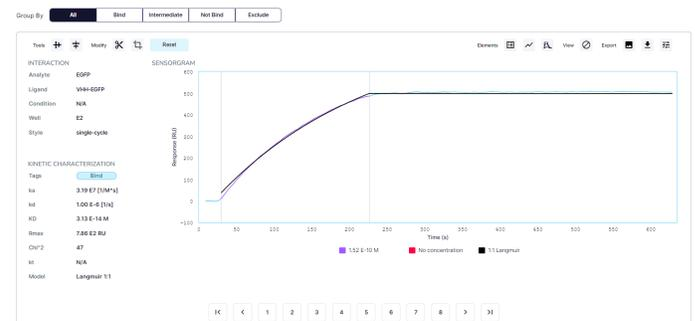
**Figure 4:** Corrected binding curve of EGFP in well E2 binding to VHH-EGFP as the ligand. The software indicates a positive binding event between EGFP (analyte) and VHH-EGFP (ligand). Using a 1:1 Langmuir model, the software generates estimates of  $k_a$ ,  $k_d$ ,  $K_D$  and  $R_{max}$  values. Image was generated by Nicosystem analysis software.
