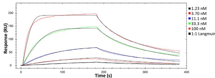
**Figure 3:** Multi-cycle kinetics of HuCAL (analyte) binding to captured GFP (ligand) on (A) Alto and (B) conventional SPR. Analyte was titrated from 1.23 nM to 100 nM. Black curve represents the Langmuir 1:1 diffusion corrected binding fit.
