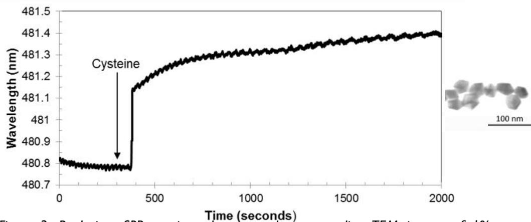
Figure 3. Real time SPR maxima changes and corresponding TEM images of 1% Au@AgDeNPs after addition of  $10^{-5}$  M cysteine. Noise less than 20 pm is achieved.
