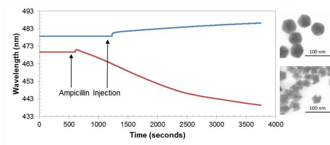
Figure 1. Real time SPR maxima changes and corresponding TEM (transmission electron microscopy) images after addition of  $10^{-2}$  M ampicillin to 1% Au@AgDeNPs and precursor AgDeNPs.
