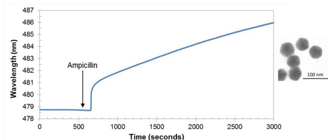
Figure 2. Real time SPR maxima changes and corresponding TEM images of 1% Au@AgDeNPs after addition of  $10^{-2}$  M ampicillin.
