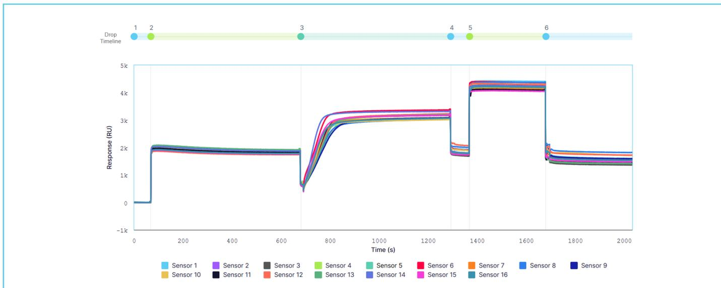
**Figure 2:** Immobilization of Strep-Tactin XT on the Alto carboxyl cartridge. The capture surface building activity includes activation of all 16 sensors with 200 mM EDC and 200 mM NHS from Nicoya's Surfacing Kit for 600 s, followed by immobilization of 5 µg/mL Strep-Tactin XT in sodium acetate pH 4.5 for 600 s, and blocking of sensors with 1 M ethanolamine for 300 s.
