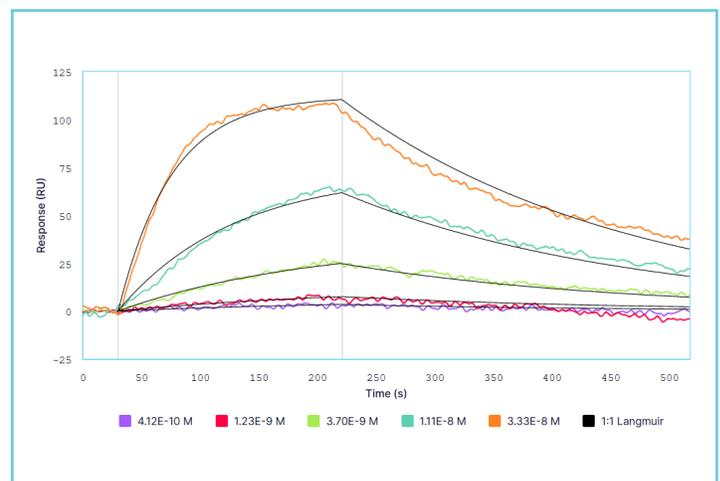
**Figure 5:** Representative sensorgram showing the binding of HuCAL to GFP-TST that is captured by Strep-Tactin XT in an MCK format. Image was generated by Nicosystem analysis software.
