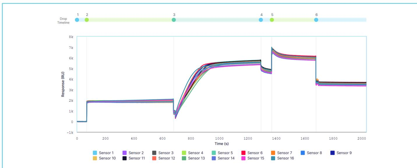
**Figure 3:** Immobilization of Strep-tag VHH on the Alto carboxyl cartridge. The capture surface building activity includes activation of all 16 sensors with 200 mM EDC and 200 mM NHS from Nicoya's Surfacing Kit for 600 s, followed by immobilization of 5 µg/mL Strep-tag VHH in MES pH 6.0 for 600 s, and blocking of sensors with 1 M ethanolamine for 300 s.
