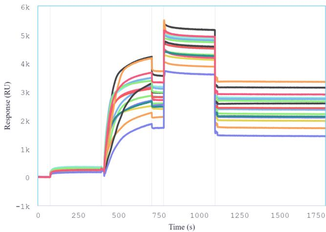
**Figure 3:** Activation of response channels with EDC/NHS from Nicoya's Surfacing Kit, followed by immobilization of 20 µg/mL of each surface antibody in Sodium Acetate pH 5.0 and blocking of sensors with 1 M Ethanolamine. Image was generated by Nicosystem analysis software.
