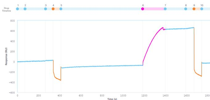
**Figure 4:** A representative sensorgram overlay showing antigen binding and then buffer in place of solution Ab. This acts as the buffer blank due to all 16 channels being used as active channels in the epitope binning protocol. Image was generated by Nicosystem analysis software.
