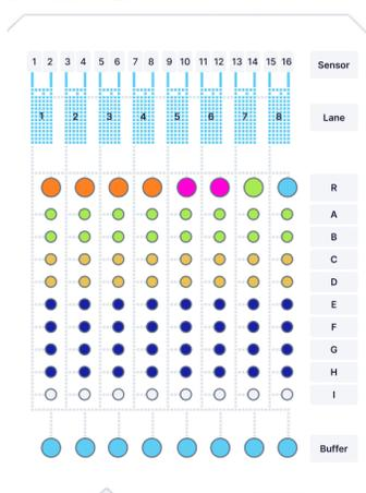
**Figure 2:** Alto cartridge layout for epitope binning reagents. Orange wells (R1-4) are regeneration solution, pink (R5-6) are antigen, green (R7, A-B) are reagents, light blue (R8 & Buffer) are buffers, yellow (C-D) are surface antibodies and dark blue (E-H) are solution antibodies.
