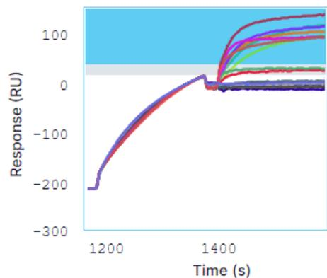
**Figure 6:** Overlay of normalized antigen binding followed by solution antibody sandwiching or blocked binding. Binding (blue region) and non-binding (white region) thresholds can be changed by the user.
