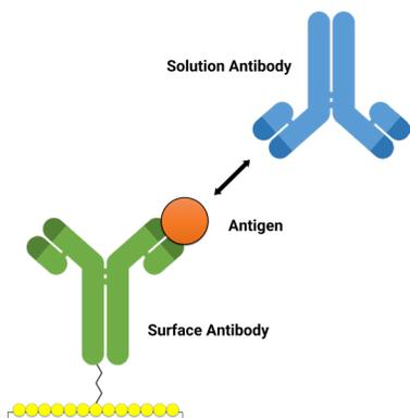
**Figure 1:** In a classical sandwich assay, the surface antibody is immobilized onto the sensor, followed by injection of the antigen and then the solution antibody. If one antibody blocks the binding of another, they can be grouped together into a bin, which indicates they compete for the same or a similar epitope.
