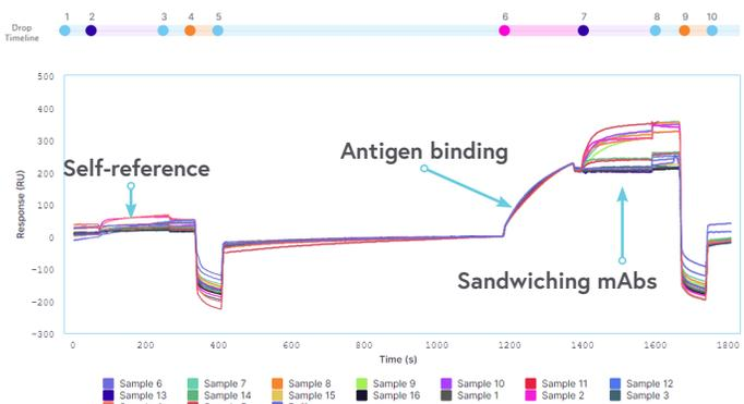
**Figure 5:** A representative sensorgram overlay showing all sixteen solution antibodies and buffer blank interacting with a single surface antibody. Solution antibody (or buffer) is passed over the sensor and used for referencing. The surface is then regenerated. This is followed by antigen, solution antibody (or buffer), and finally a second regeneration. Image was generated by Nicosystem analysis software.
