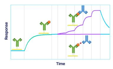
Figure 3: Epitope characterization showing capturing of the influenza A HA antigen to the immobilized surface HA antibody (green curve) followed by binding of the five automated 3-fold serial dilutions of the solution antibody to a different epitope of the antigen (top purple curves). A lack of binding of the five automated 3-fold serial dilutions of the solution antibody indicates epitope overlap of the surface antibody (bottom purple line).
