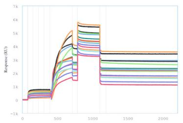
Figure 2: Surface antibody immobilization: Activation of response channels with EDC/NHS from Nicoya's Surfacing Kit, followed by immobilization of 20  $\mu$ g/mL of each surface antibody in Sodium Acetate pH 5.0 and blocking of sensors with 1 M ethanolamine. Image was generated by Nicosystem analysis software.
