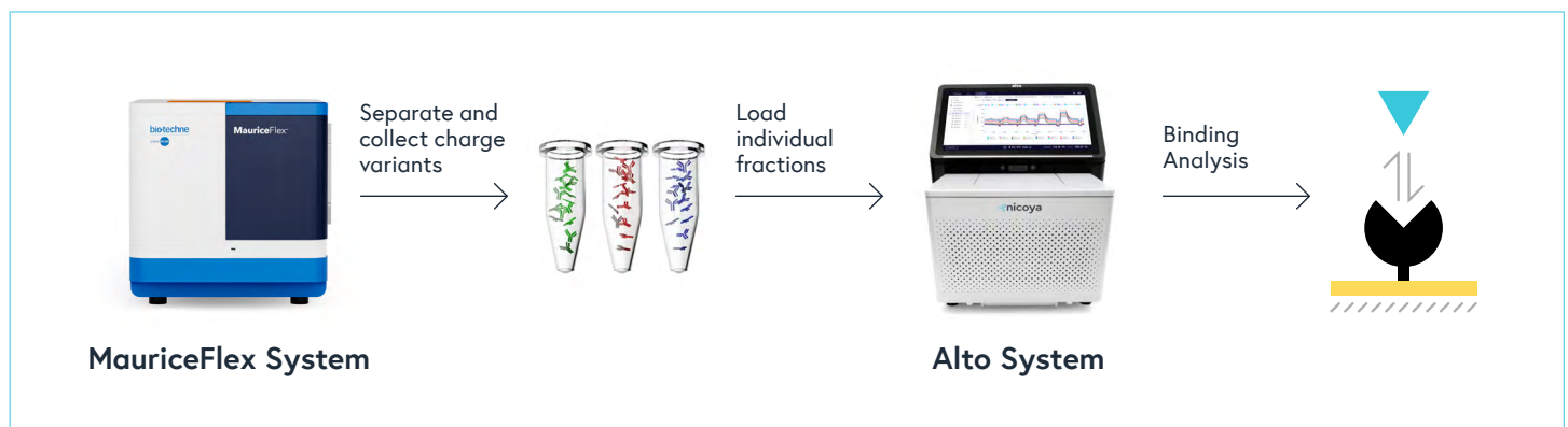
Figure 1: Biotherapeutic charge heterogeneity analysis and charge variant fraction collection workflow with the MauriceFlex System, followed by binding analysis on the Alto System.
